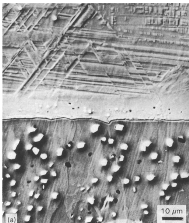
Figure 3 Interface morphologies for the couples in series I, diffused at 1000 °C for 158 h: (a) H/C, (b) H/D, (c) H/E, and (d) H/F.
